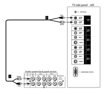
Figure 7. Connecting the Stereo Audio System.
